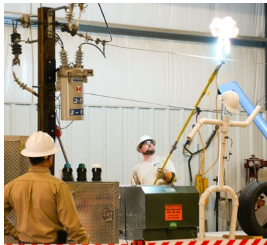
JR Hynek creates a bright arc demonstrating the dangers of coming into contact with a power line
